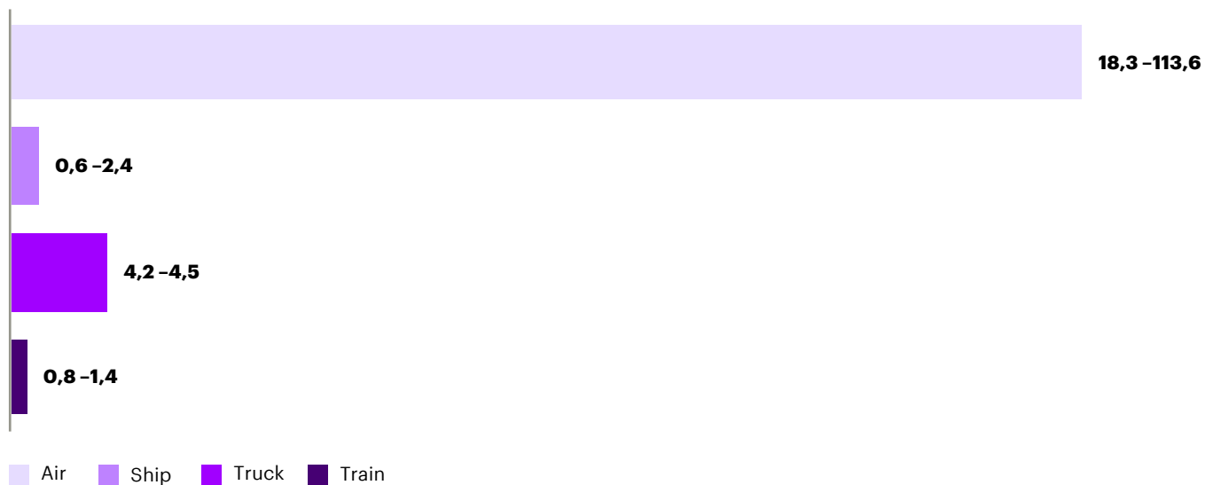
Figure 3: Average energy consumption for different freight transport modes – simplified 5
