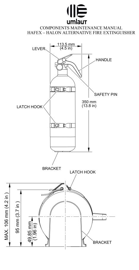
COMPONENTS – HAFEX - HALON ALTERNATIVE FIRE EXTINGUISHER FIGURE 2/GRAPHIC 26-24-01-991-002-A01
