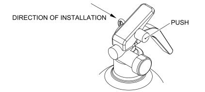
SAFETY PIN INSTALLATION FIGURE 6002/GRAPHIC 26-24-01-991-016-A01
