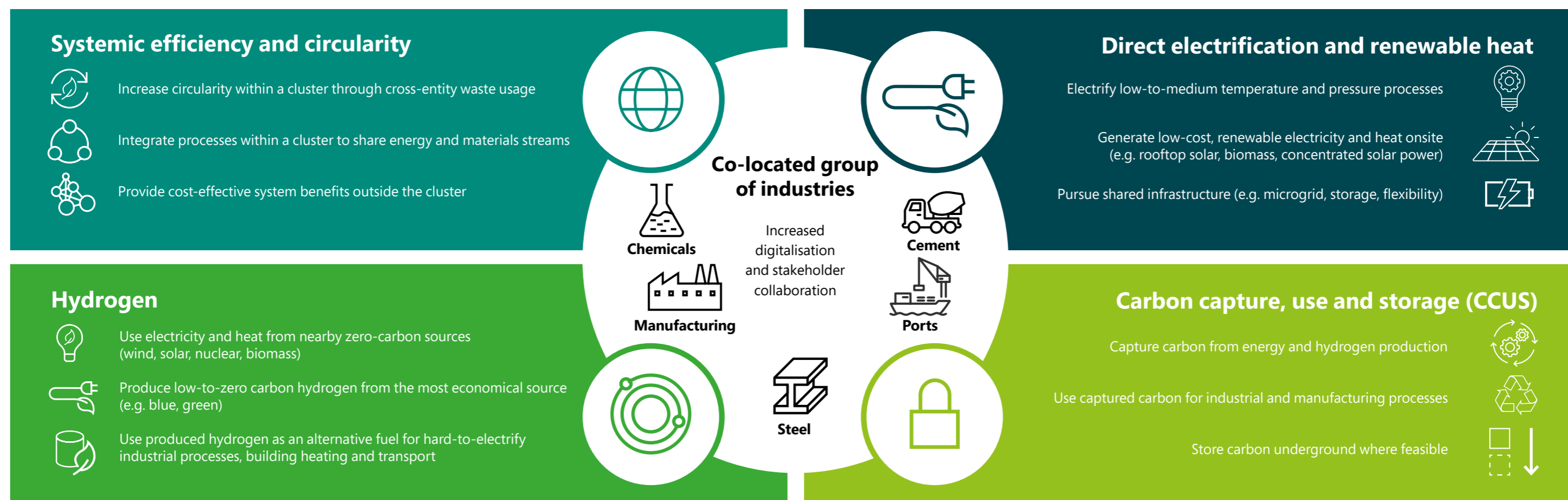
Figure 2. Emissions-abatement options for industrial clusters. To minimise emissions and design an integrated energy system with optimal value outcomes, it is best to consider the cluster as a whole.
