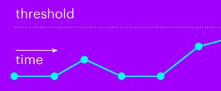
A neuron receives input signals from sensors and other neurons over time. The neuron adds the inputs to its membrane potential (V) and subtracts a fraction of the value from the previous timestep (leak). If the integrated input values are large enough, V exceeds the threshold, causing the neuron to fire an output spike and reset V back to zero.
