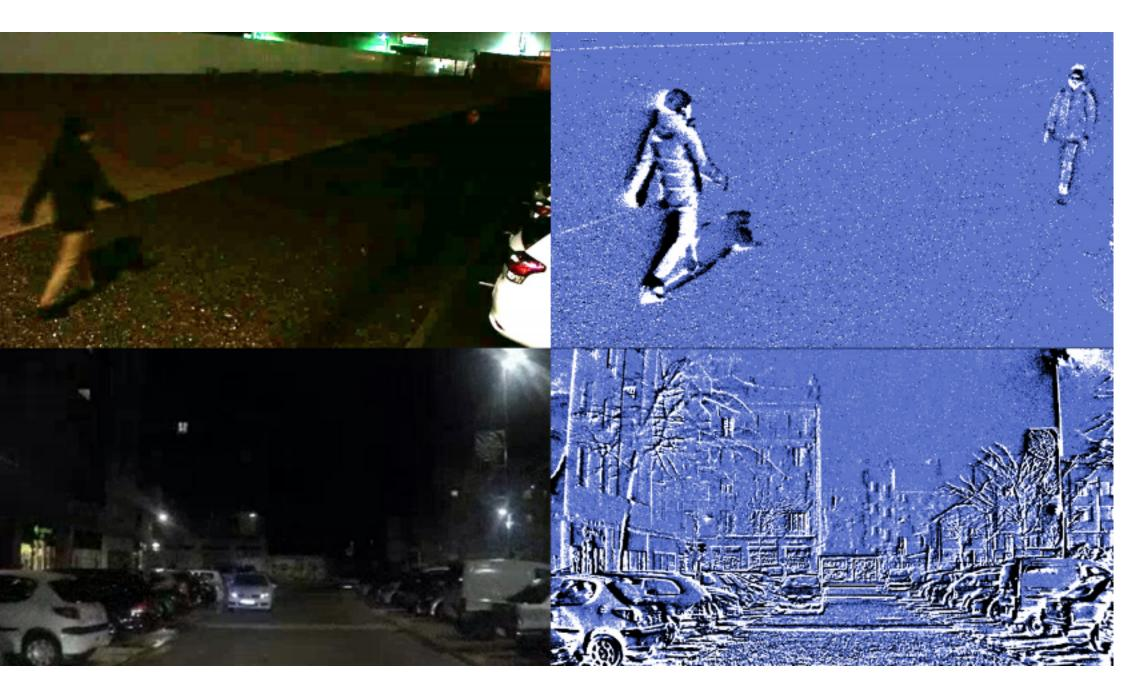
The event-based sensor (right) records only when a scene changes. This generates less data, improving energy efficiency and reducing latency in addition to generating more contrast. In the top images, pedestrians passing in front of the sensor are clear even with minimal ambient light. In the bottom images captured from a moving vehicle, the outlines of all relevant objects are distinctly visible. (Images courtesy of Prophesee)
