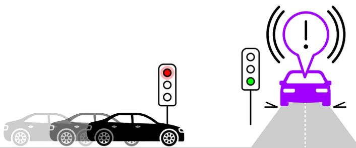
A smart car prevents a possible accident by quickly edge processing and analyzing its own speed, the speed of the upcoming car, and both of their locations, and hitting the automatic brakes.
