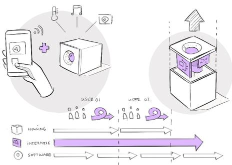
Video baby monitor fully optimized for material use reduction, power consumption reduction, refurbishment and upgradability.
