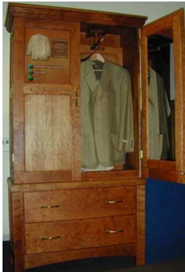
Figure 3. As a physical interface to online stores, ONLINE WARDROBE has a built-in touch sensitive LCD, voice output, and an RFID sensor for detecting its contents.
