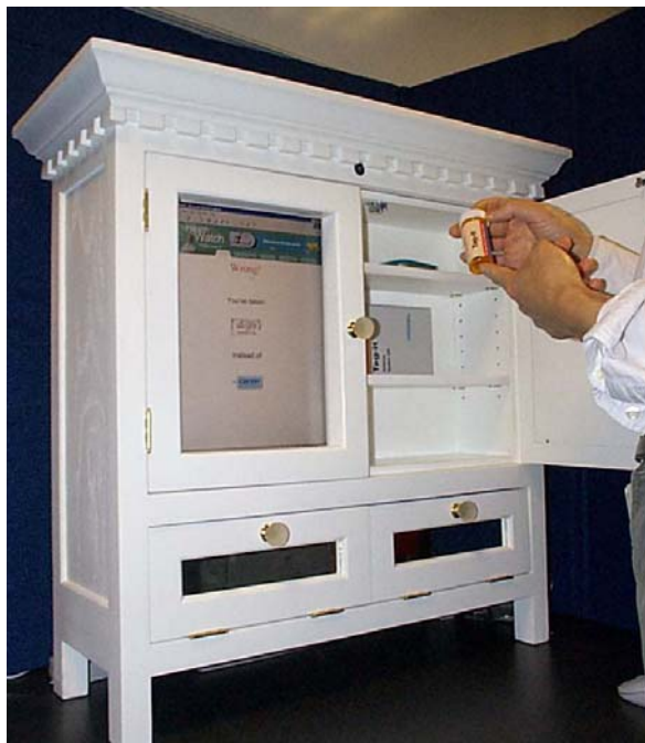
Figure 1. MMC knows what medication is in the medicine cabinet, and warns you if you accidentally pick up the wrong bottle.
