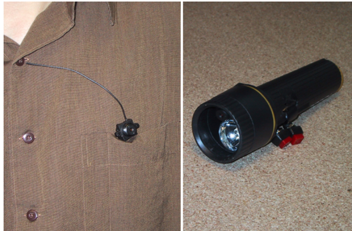
Figure 6. On the left, a 900 MHz wireless camera (courtesy of Super Circuits, Inc.) in a shirt pocket allows hand-free operations. On the right, the flashcam has built-in flashlight, wireless camera, and laser pointer.
