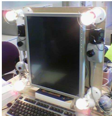
Fig. 3. Components of the digital mirror: two cameras, one touch screen and some lights.
